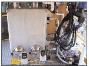
Top: The locomotive on the TDC evolution has good visibility forward for spraying the ballast Middle: Spraying equipment is extremely flexible, with varying combinations of herbicide able to be sprayed simultaneously, all controlled from a single panel.
