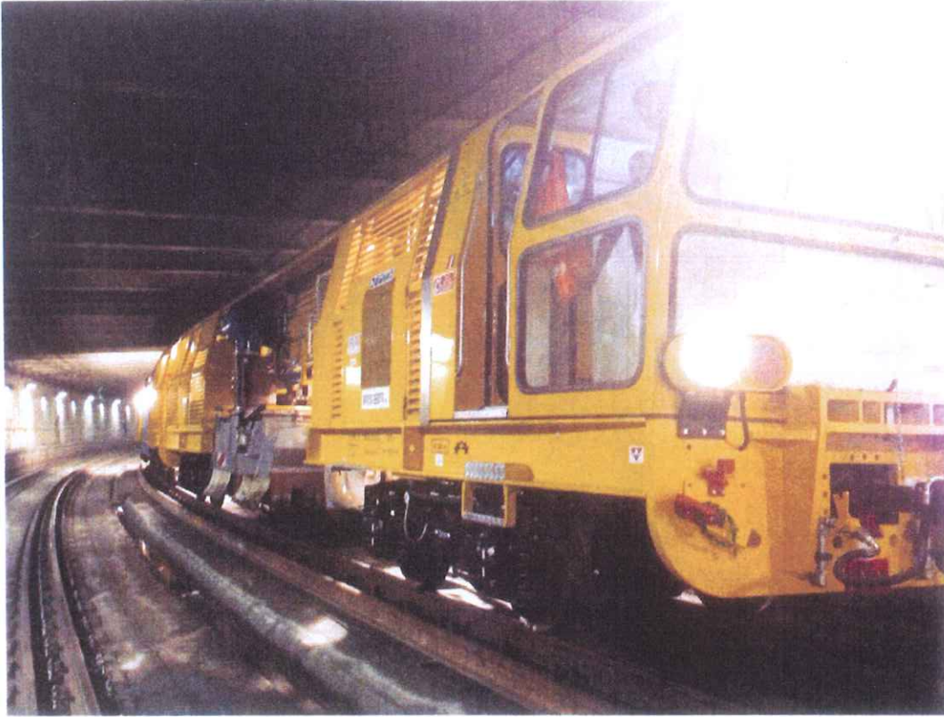
The SAI 400 EVO de-dusting train was developed from similar machines used in main line tunnels.
